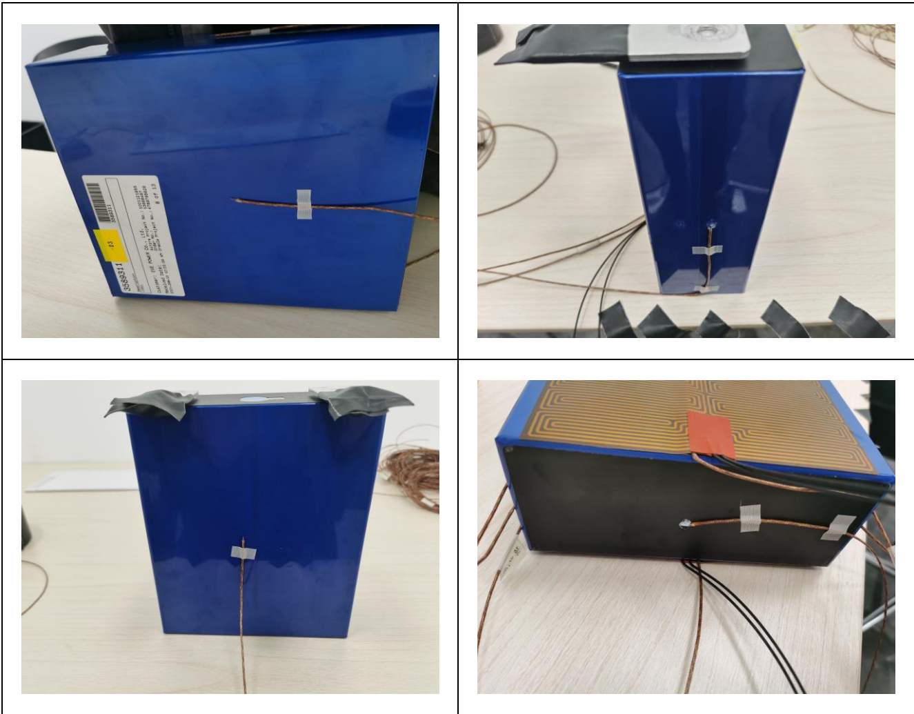
Figure 7: Sample 2 Instrumentation Prior to Test Note: heaters were placed on two sides of cell after thermocouple adhered.
